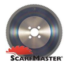
The PVD coated carbide tipped ScarfMaster has specifically been designed for flying cut-off applications dealing with heavy inside scarf. It features a very specific tooth geometry, combined with highly shock resistant carbide tips.
