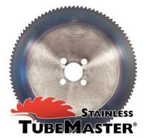
The TubeMaster Stainless saw blade has specifically been developed for cutting stainless steel tubes on orbital flying cut-off units. These saw blades can cope with cutting speeds between 60 - 120 m/min. TubeMaster Stainless offers high uptime due to a blade life up to 3.5m², combined with high cut quality and production output.
