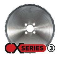
The CX3saw blade has been developed for cutting tubes on high performance automatics awing machines, at a higher maximum cutting speed than possible with HSS saw blades. It is most effective on sawing machines with accurate control of chip load and variable feed rate. Bigger tips are applied at pitches > 9mm for added stability.
