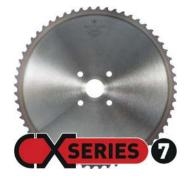
CX 7 is a Cermet tipped, PVD coated saw blade dedicated to cutting carbon steel (carbon content < 0.60%) with a low to medium tensile strength up to  $750 \text{ N/mm}^2$ . The best blade performance is being achieved when cutting lower tensile materials. On many applications, a blade life of  $50 \text{ m}^2$  and more can be achieved.
